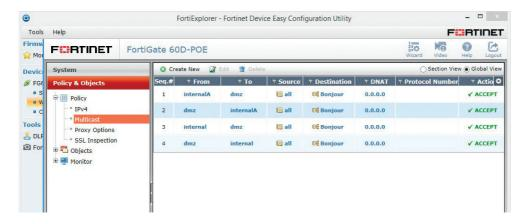
18. As mentioned earlier, the Time To Live (TTL) value for each package is very important. Our entire AirPlay/ Bonjour package should pass through the firewall unaltered. To enable this, we will first have to enter some CLI commands into the firewall.
