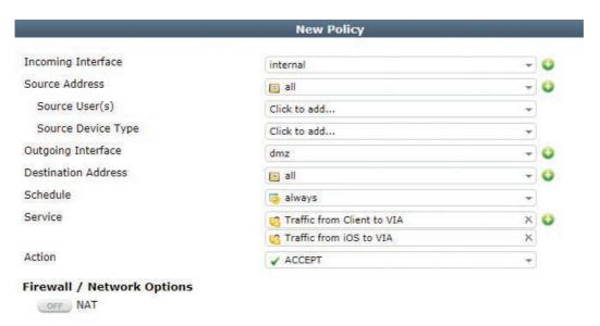
28. Finally, create a policy to allow communication back from DMZ to internal.
