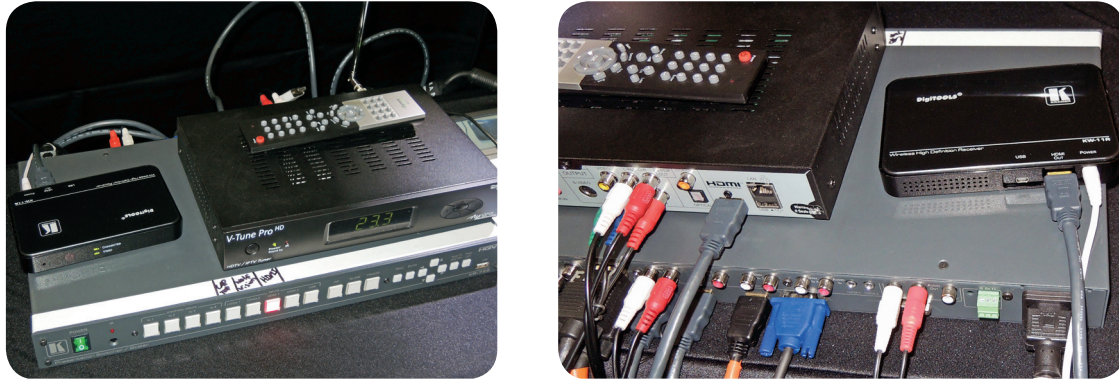
Figure 5. The KW-11 provides a wireless HDMI input to a Kramer VP-728 ProScale™ presentation scaler/switcher
