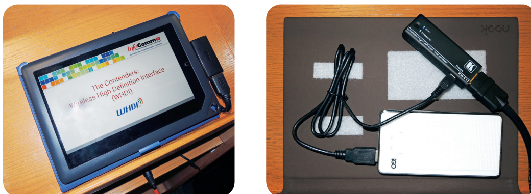
Figure 4. This wireless Nook tablet uses the KW-11 stick and a high-capacity iGo battery for power
