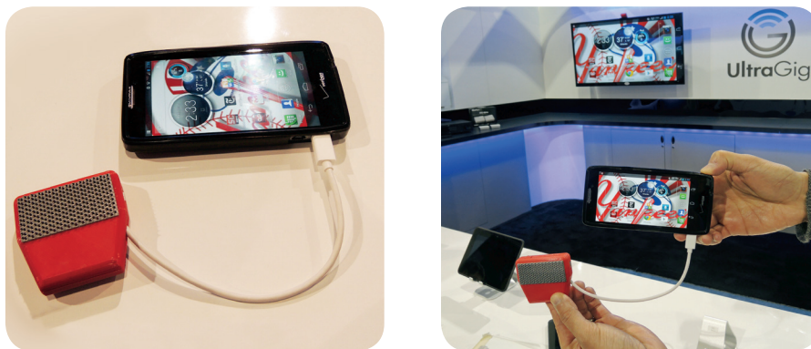
Figure 2. A WiHD prototype dongle, streaming 1080p/60 content from a smartphone to a nearby TV
