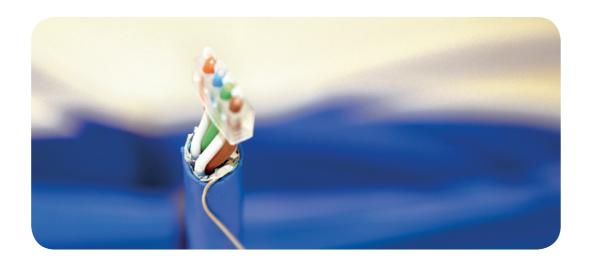
**Step 8:** Using the standard crimp tool, crimp the RJ45 connector.
