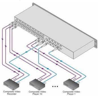
Figure 5: Connecting the VS-101AV
