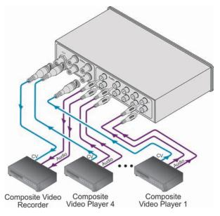
Figure 4: Connecting the VS-41AV
