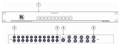
Figure 2: VS-101AV 10x1 Video/Audio-Stereo Switcher
