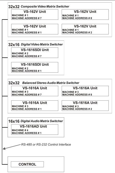
Figure 11: Assembling a System of Interconnected Switchers
