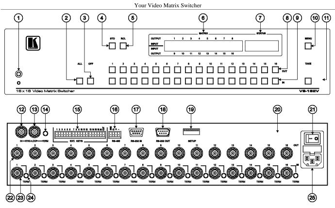
Figure 1: VS-162V 16x16 Video Matrix Switcher
