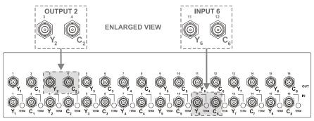
Figure 4: Configuring the VS-162V for s-Video (Y/C)
