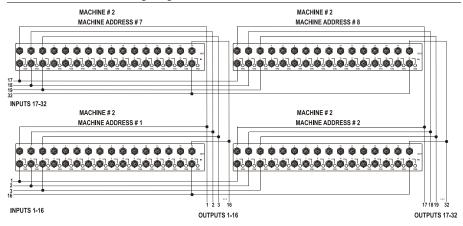
Figure 10: Connecting the 32x32 Switcher
