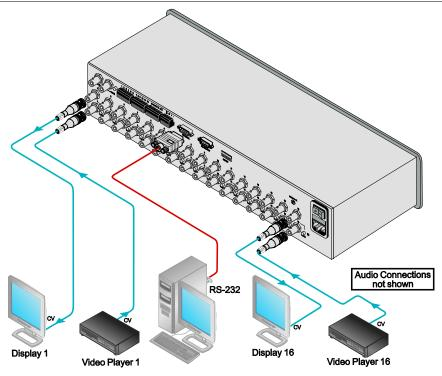
Figure 3: Configuring the VS-162V for Composite Video (CV)
