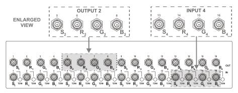
Figure 6: Configuring the VS-162V for RGBS
