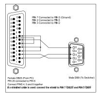
Figure 14: Connecting to a 25-pin PC COM Port without a Null-Modem Adapter
