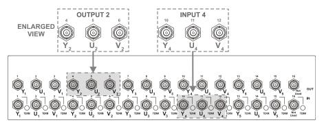
Figure 5: Configuring the VS-162V for YUV (RGB)
