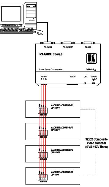
Figure 17: An RS-485 Control Interface Setup
