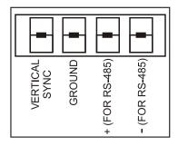
Figure 15: RS-485 Connector PINOUT
