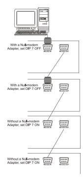
Figure 13: Connecting a PC to 4 VS-162V Units
