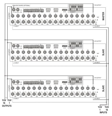
Figure 7: Configuring a 16x16 YUV (RGB) Switcher with 3 VS-162V Units
