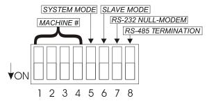
Figure 12: Rear Panel DIP-switches
