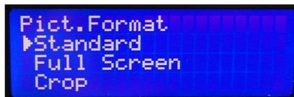
a. **Standard** displays your input signal pixel for pixel, it preserves the size and aspect ratio of the incoming image. Areas of the display that are un-used are displayed black (letterboxed).
