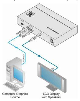
Figure 2: Connecting the VP-506 DVI/UXGA Scan Converter
