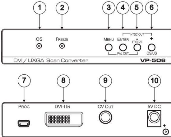
Figure 1: VP-506 DVI/UXGA Scan Converter
