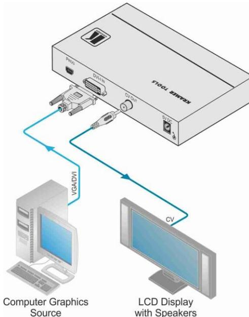
Figure 2: Connecting the VP-506 DVI/UXGA Scan Converter
