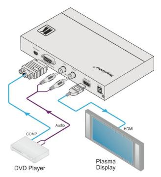
Figure 2: Connecting the VP-425 PC / Component to HDMI Scaler
