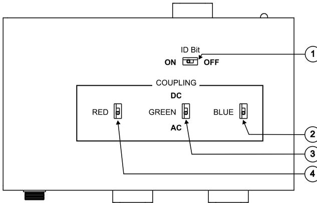
Figure 4: VP-200XLN XGA Line Amplifier / DA (Underside)
