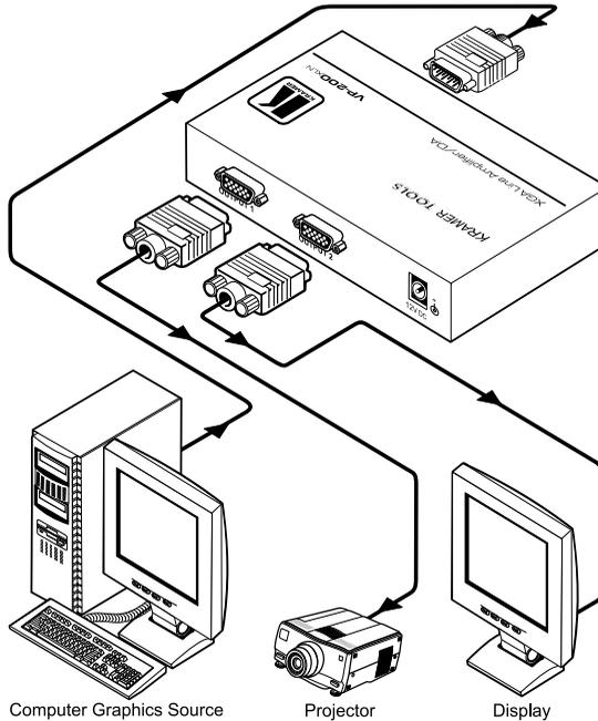
Figure 5: Connecting the VP-200XLN XGA Line Amplifier / DA
