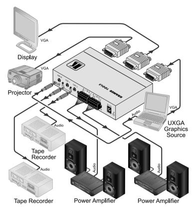
Figure 2: Connecting the VP-200AK 1:2 UXGA / Audio DA
