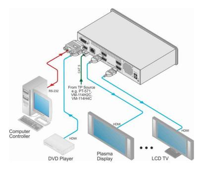
Figure 2: Connecting the VM-114H 2x Input 1:4 HDMI DA
