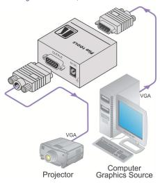
Figure 3: Reconnecting the Display Device
