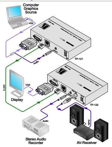
Figure 13: Connecting the XGA/Audio Line Transmitter/Receiver System
