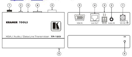
Figure 9: TP-123 XGA/Audio/Data Line Transmitter
