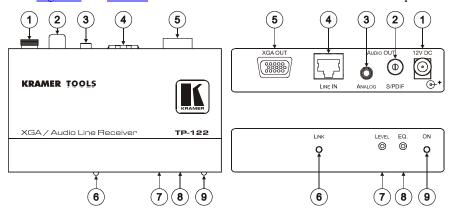
Figure 7: TP-122 XGA/Audio Line Receiver (Topside)
