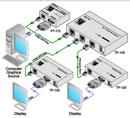
Figure 18: Configuring a TP-105 CAT 5 Line Driver/DA
