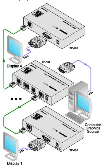
Figure 17: Configuring a 1:4 XGA to Twisted Pair Transmitter/Receiver/DA
