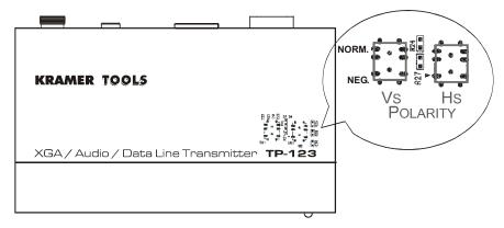
Figure 10: TP-123 Internal Polarity Switches
