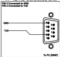
Figure 16: RS-232 PINOUT Connection
