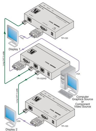
Figure 3: Configuring a 1:2 XGA/HD to Twisted Pair Transmitter/Receiver/DA
