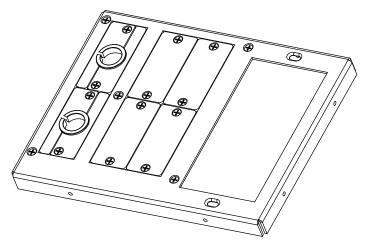
Figure 10: Cable Pass-through Insert (P/N: 80-000399)
