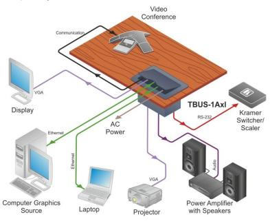
Figure 11: TBUS-1Axl Boardroom Installation
