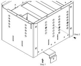
Figure 5: Installing the T-TBLANK TOOL Blank
