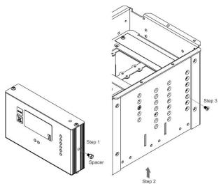
Figure 4: Installing a Kramer TOOL
