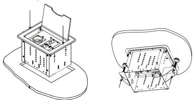
Figure 9: Inserting TBUS-1Axl into the Prepared Opening
