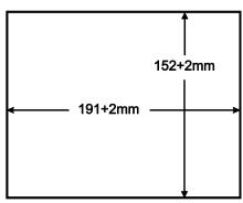
Figure 8: Cut out Dimensions
