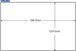
Figure 4: Cut out Dimensions
