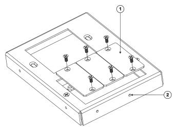
Figure 3: TBUS-5xl Inner Frame (P/N: 80-004099)
