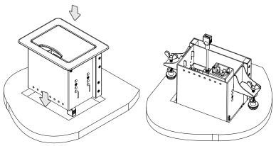
Figure 5: Inserting TBUS-5xl into the Prepared Opening
