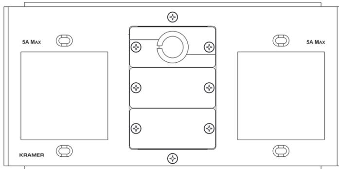
Figure 1: T4F-23 Inner Frame (P/N: 80-003699)
