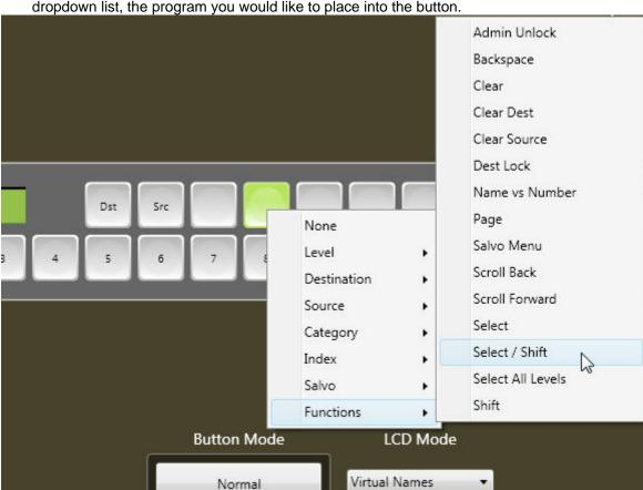
To program a button hover over the button with the mouse pointer, right click, and select from the dropdown list, the program you would like to place into the button.
