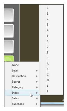
**<u>Destination</u>**; This is a list of outputs, by name, providing a direct routing path to a selected output.
