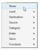
**Level**; This list contains the levels of control active on the router. When this function is applied to a panel button the LED for that button will light allowing individual level selection. After a destination is selected all level buttons will light. Pressing a level button will unselect the level indicated by extinguishing the light. Holding down the button will cause the panel to cycle from enabling only the level selected to all levels enabled.
