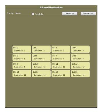
All control panels can have outputs blocked, this allows the control panel to status an output, but prevents the panel from selecting inputs on that output.
