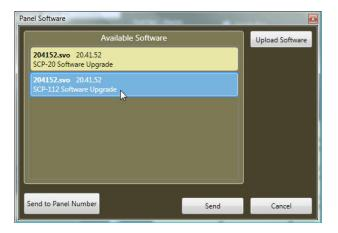
The panel's software upgrade process will be indicated on the LCD screen of the panel by "Receiving Text #####". The panel will reset when transfer is complete.
