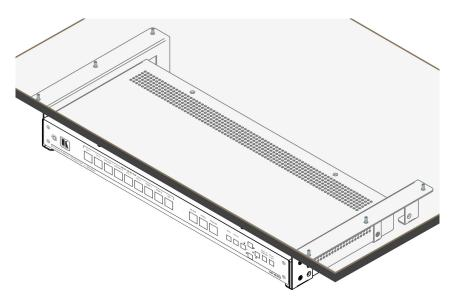
Figure 2: RK-19 Installed under a Table
