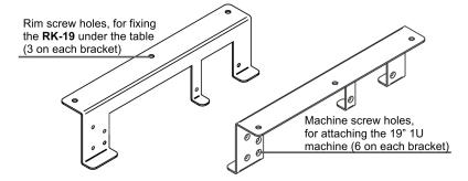
Figure 1: RK-19 Under-the-table Brackets
