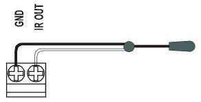
Figure 4: IR Emitter Wiring
