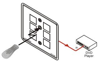
Figure 5: IR Repeater Operation
