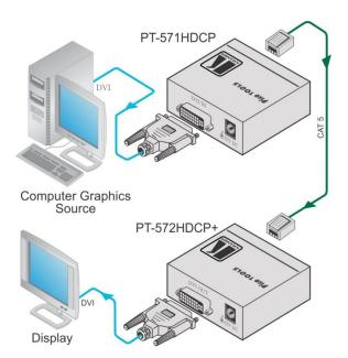
Figure 3: Connecting the PT-571HDCP/PT-572HDCP+ Transmitter/Receiver Pair
