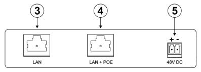
Figure 2: PSE-1 10G POE Injector Rear Panel
