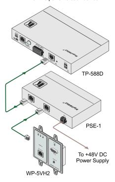
Figure 3: Connecting the PSE-1 10G POE Injector
