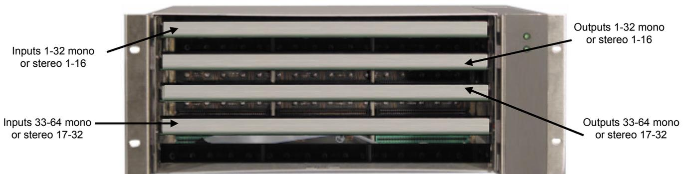
The top slot in both the analog and digital frame contains the input buffer module for inputs 1-32.
