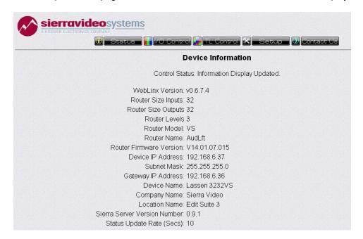
To setup IP address parameters, select "Setup".
