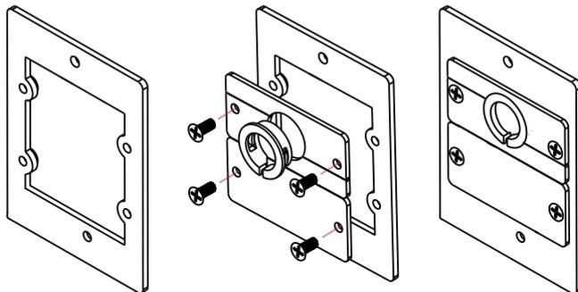
2. Connect the cable ports to the rear side of the insert(s).
