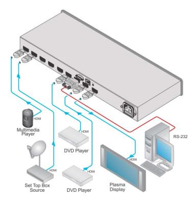
Figure 3: Connecting the VS-81H 8x1 HDMI Switcher
