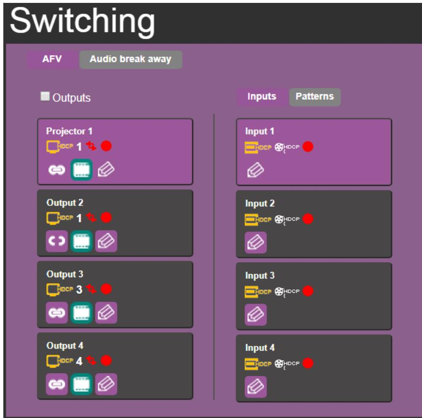
Figure 20: Switching Page – AFV Tab
