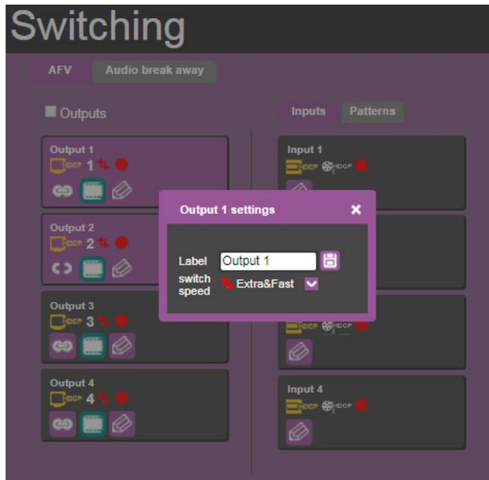
Figure 15: Switching Page – Editing the Output Button Settings
