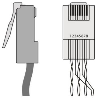
The image shows a side view of an RJ-45 connector on the left and a wiring diagram on the right. The wiring diagram shows a rectangular connector with eight pins labeled 1 through 8. Below the pins, the numbers 12345678 are printed. Eight wires are shown extending from the bottom of the connector, each connected to a corresponding pin.
