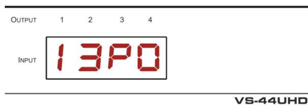
In this example: Input 1 is routed to output 1, input 3 is routed to output 2, a pattern is routed to output 3, and output 4 is set to mute.
