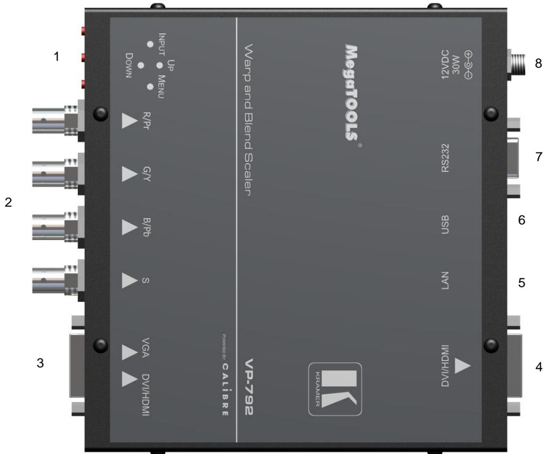
1 – Keypad with three keys for OSD menu navigation (Menu, Down and Up) and a key for input channel selection (Input).
