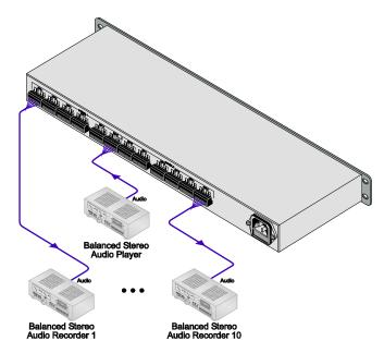
Figure 3: Connecting the VM-1610 in a 1:10 Configuration
