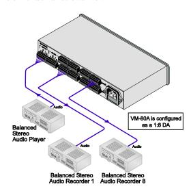
Figure 4: Connecting the VM-80A in a 1:8 Configuration
