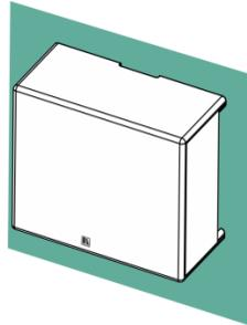
On the floor vertically with woofer facing the wall and the bass port facing the floor.
