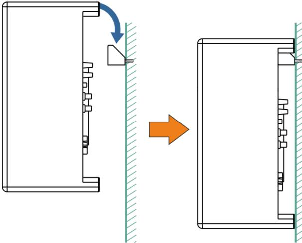
Figure 9: Mounting Tavor 8-Sub over the Bracket
