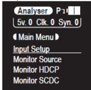
The status line displays the 5V, TMDS clock, and sync detection state of the connected source (1 = detected, 0 = not detected).
