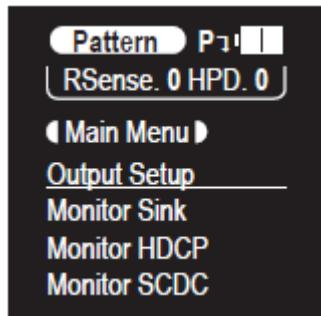
The status line displays the RxSense and Hot-plug detection state of the connected display (1 = detected, 0 = not detected).
