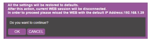
Figure 25: Device Settings Page - Factory Reset
