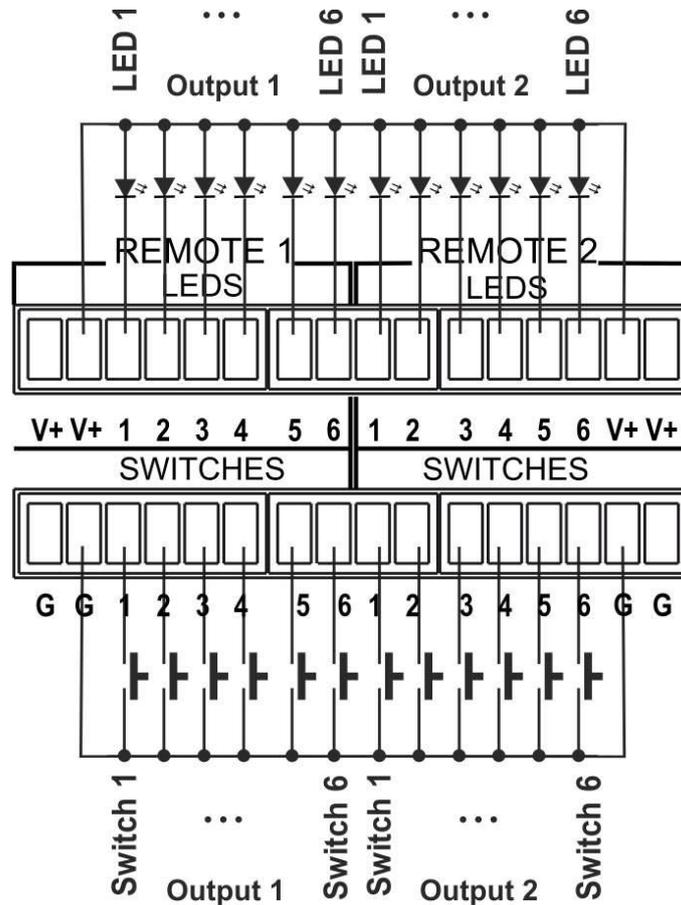
Figure 7: Remote Contact-closure Switch and LED Connections
