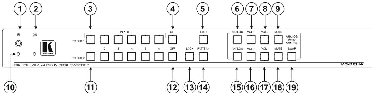
Figure 1: VS-62HA 6x2 HDMI/Audio Matrix Switcher Front Panel
