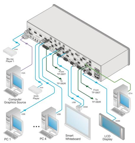
Figure 3: Connecting the VP-558 Presentation Switcher / Scaler
