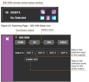
Figure 25: Switching Page - SID-X2N Setup Window
