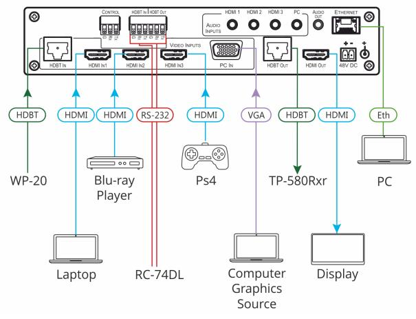
Figure 3: Connecting to the VP-440H2 Rear Panel
