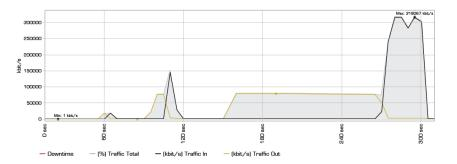
The graph below shows a series of files (10MB, then 100MB, then 1,024MB) uploaded by a computer with a gigabit Ethernet connection and then downloaded by a computer with a 100 Mbps connection.
