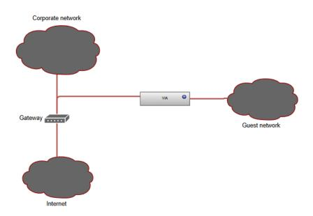
In this scenario, VIA is connected to both a corporate network (LAN 1) and a guest network (LAN 2). The corporate network is configured to assign a DHCP address with all related information. The guest network is not used by VIA to gain internet access or resolve domain names but is also configured to assign a DHCP address.
