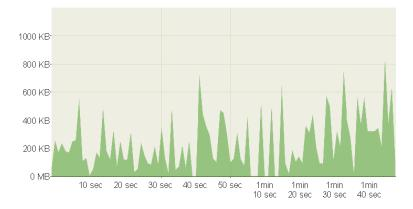
Slides with text and a few graphics are displayed on the **VIA** main display by a single connected client. Slides were advanced in irregular times to simulate real workflow.
