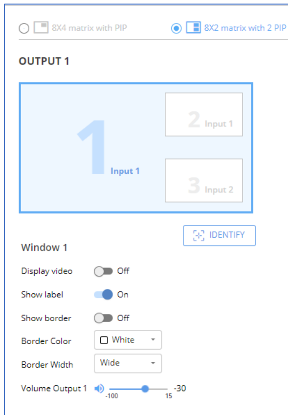
Figure 35: 2 PIP (8X2 Matrix) Layout – Window 1 Parameters Settings
