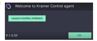
b. Press Launch Control Interface and enter the IP address and port of the interface you defined in Kramer Brain, for example "https://<Brain-IP>:8001". The hardware section of the builder's Brain info contains the IP:port# of the Brain.
