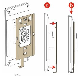
5. Insert one M2.5 screw below the touch panel and secure the touch panel to the wall mount bracket.
