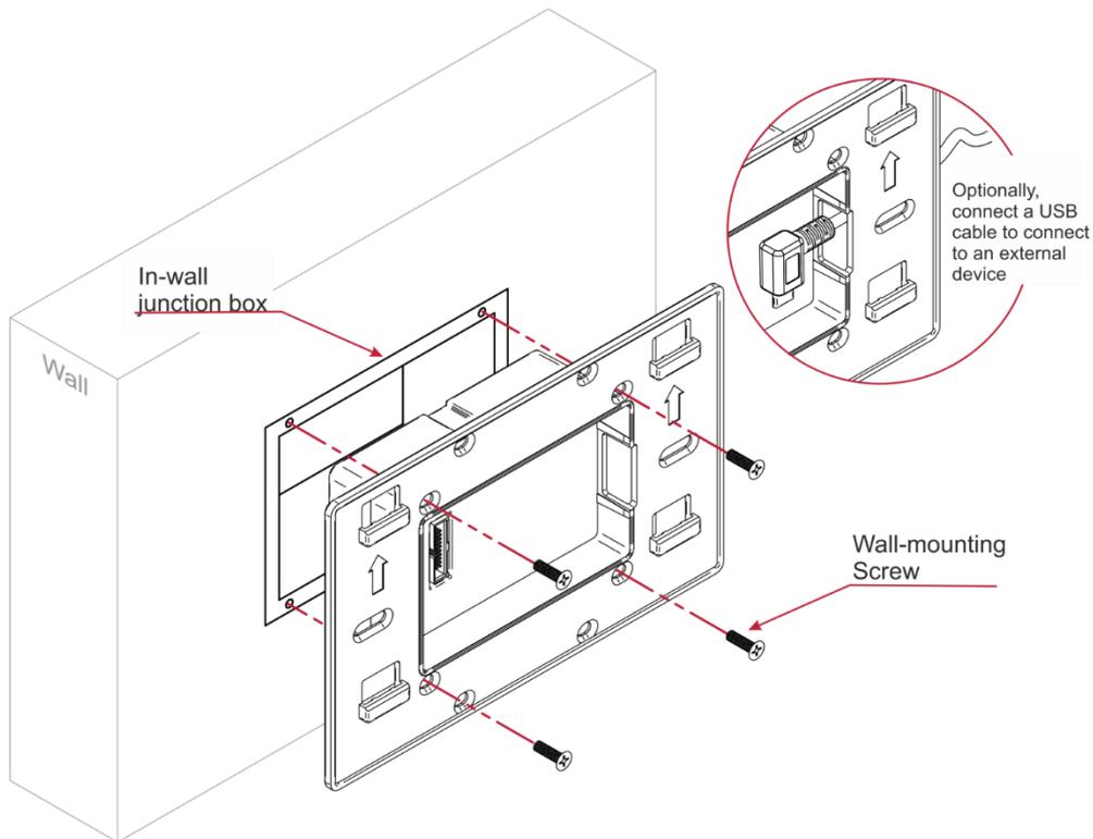
Figure 10: Installing the On-Wall Mount Unit
