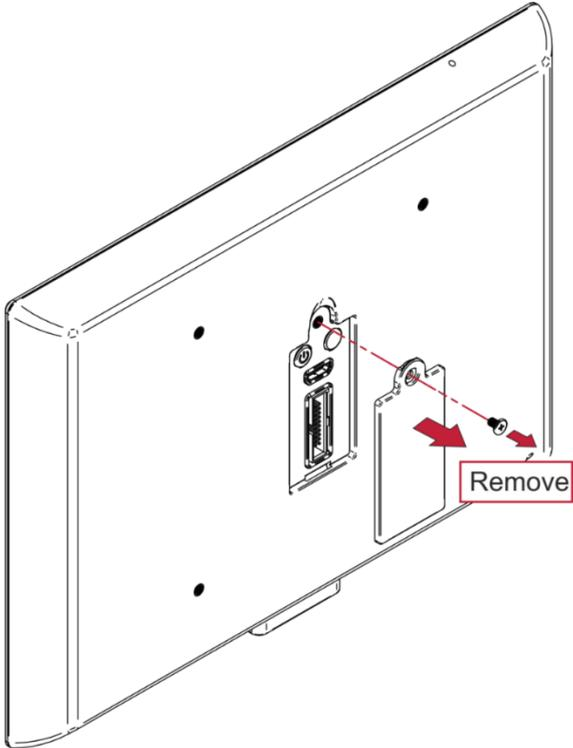
Figure 11: Removing the Cover on the **KT-107S** Rear Side
