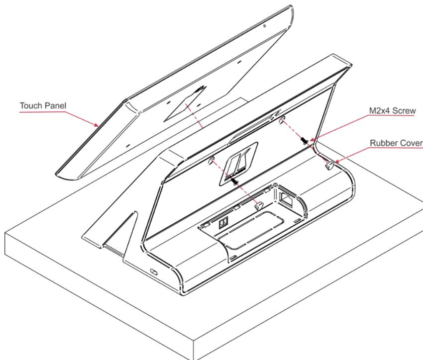
Figure 8: Connecting to the KT-107S Rear Panel
