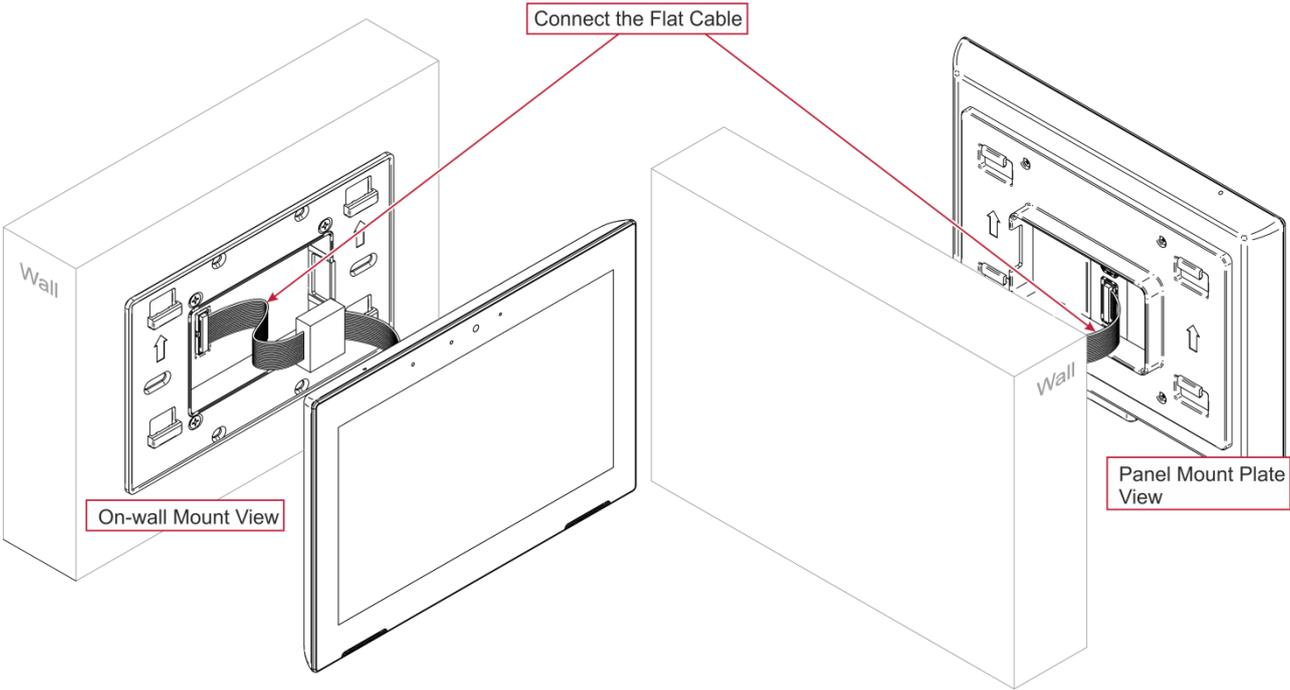
Figure 13: Connecting the On-wall Mount Flat Cable
