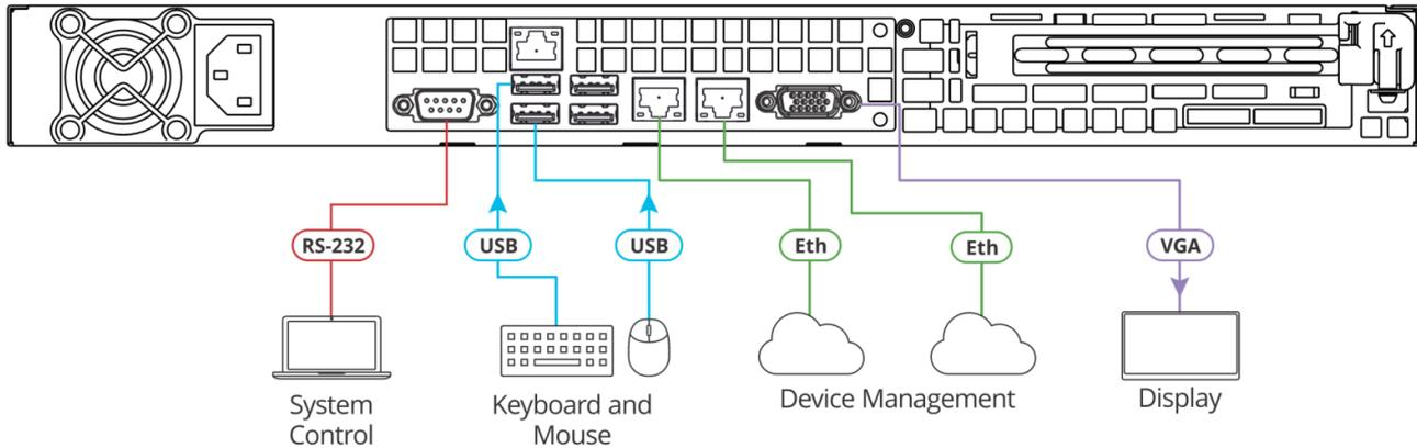
Figure 2: Connecting to the KN-100 Rear Panel
