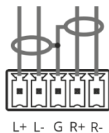
Figure 4: Connecting to a Balanced Stereo Audio Source/Acceptor
