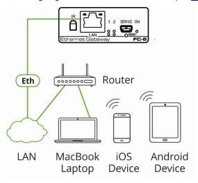
Figure 3: Connecting the FC-6 for Initial Configuration
