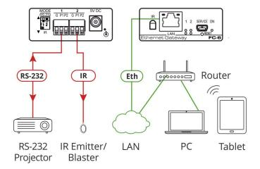
Figure 1: FC-6 Controlled Devices from Remote IP-based Clients
