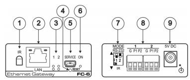
Figure 2: FC-6 Ethernet Gateway - RS-232/IR
