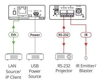
Figure 5: Connecting the FC-6 Ethernet Gateway - RS-232/IR
