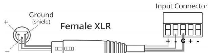
Figure 3: Connecting a Balanced XLR Input
