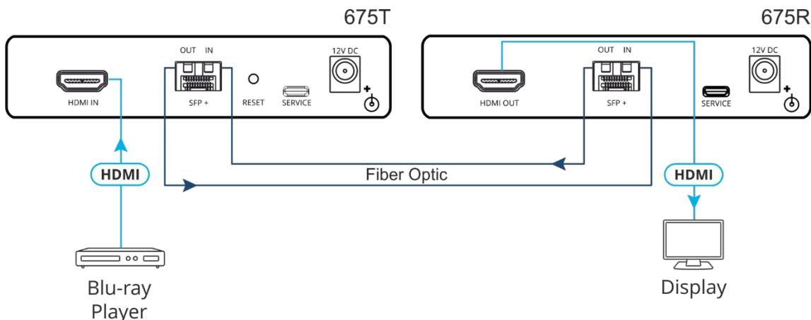
When using a duplex OSP SFP+ transceiver, connected with 2 fiber strands, always cross-connect the fiber connections, Rx OUT to Tx IN and Rx IN to Tx OUT, as unidirectional optical transmission is carried on simplex fiber strands.
