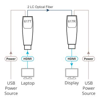
Once the system is connected the Status LEDs on both 617T and 617R flash.
