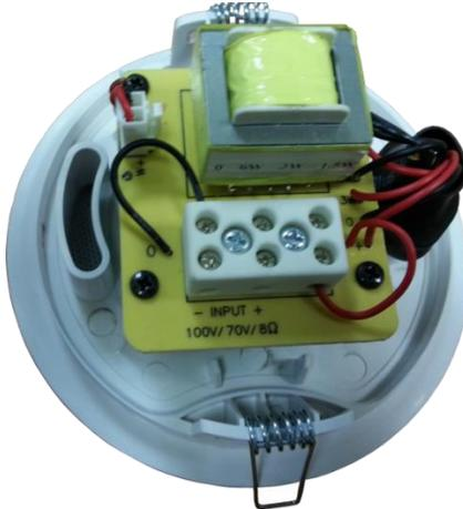
Figure 4: Ceramic Terminal Pinout
