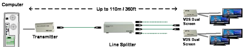
Figure 2: Expanded VGA Extender System Overview
