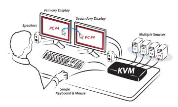
HSL Dual-Head 4-Port KVM Switch System Diagram
